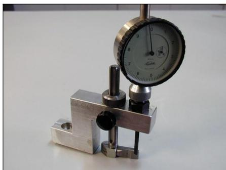
**KIT BOMBA-INYECTOR DETROIT DIESEL TIPO 5236991**
