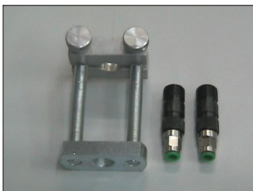
Clamps Kit to detect on test bench delivery Common-Rail injectors, by a pressurized measurement P.N.: KIT-MRS1*
