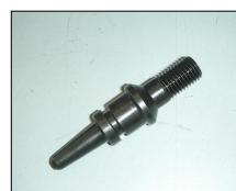
Needle for injector gau- ge block P.N.: 555-41/U
