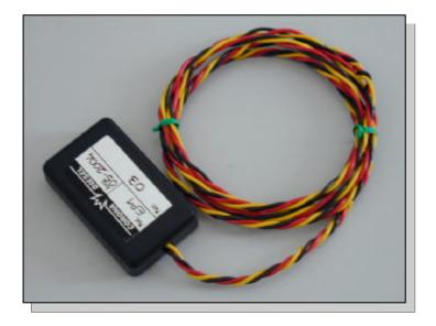
Turbo pressure emulator, using the 5 V c.c pressure sensor permits an electronically controlled system to work at a pressure which is higher than the nominal and without recording a defect code
