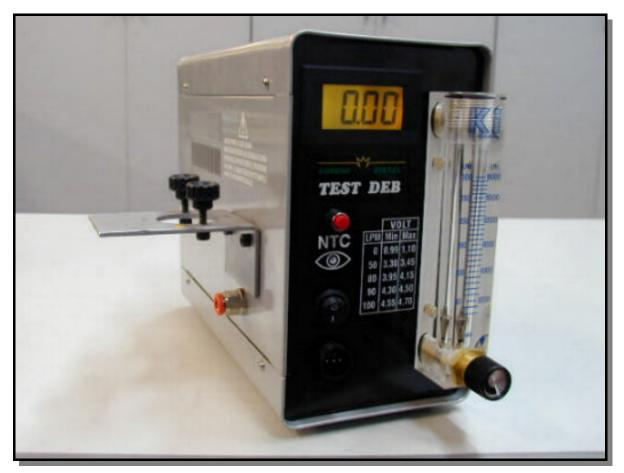
With "TEST-DEB" the efficiency of Bosch hot film (**A**, **B** type) air mass-meter can be easily measured (and backtested) this is achivied throught an air flow adjusted by a flow meter imposted over the reading lamella.
