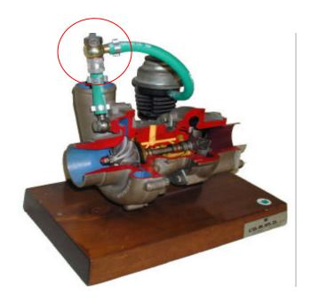
Turbocharger pressure is adjustable by a screw on the Over-Boost.
