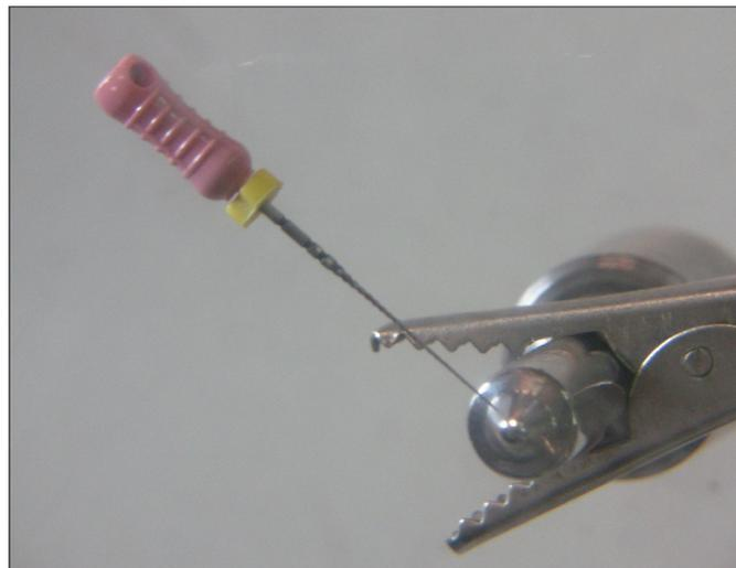
Nozzle holes, especially those from common-rail are so small that can easily get damaged on their outer part; since the hole becomes less wide fuel delivery may be affected. **FRS02** milling cutter is designed to remove leak particles and restore nozzle hole to its earlier condition.
